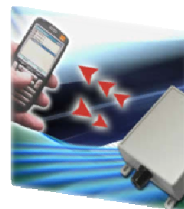
Fig 1 Shared Frequency Band. The frequency-hopping Bluetooth and fixed-frequency Wi-Fi wireless networks share a frequency band, which will result in packet collisions when the Bluetooth frequency falls within a Wi-Fi channel.
